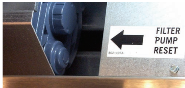
Reset switch location: New-style FPIII
